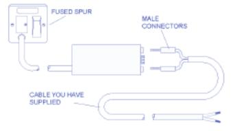
6. Push in the connectors to the transformer terminals and connect the other end of the cable to the terminals on the back of the product.
