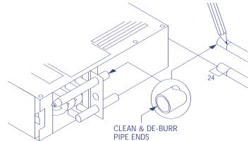
3. Connect the flexible hoses (the ends that include the isolating valves) to the heater flow and return pipes. Connect the other ends of the flexible hoses to the heating system flow and return pipes. If the connections are correct the marks you made on the pipes will NOT be visible. Open the valves and check for leaks. To remove the flexible hoses see page 23.
